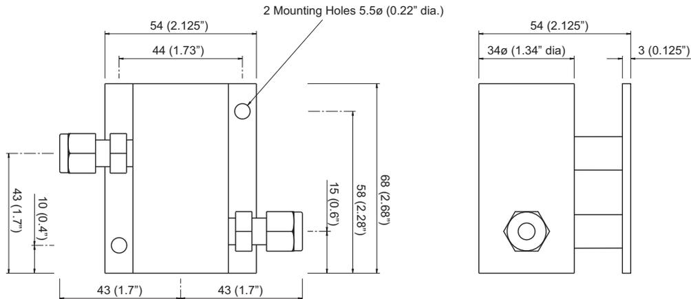
Note: The Assembly is shown with 1/4" OD tube fittings. The dimensions across the tube fittings will vary for all other size fittings.
